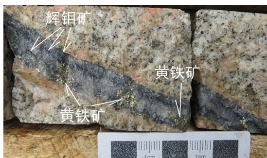
Figure 10. The edge of the vein body are filled with molybdenite, the holes in the vein body are filled with pyrite
