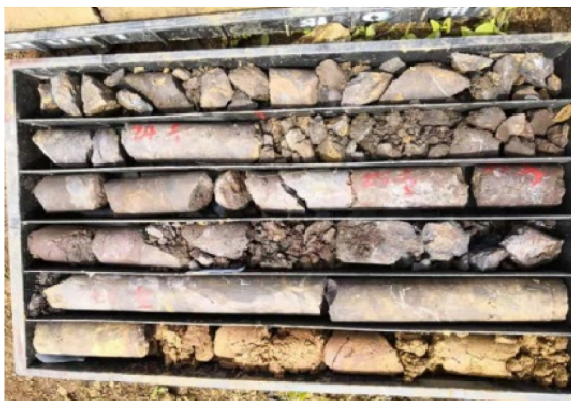
Figure 8. The bottom of Fe-Mn mineralization layer is mudstone (data source: The Third Institute of Geological Engineering Investigation of Shanxi Province)
