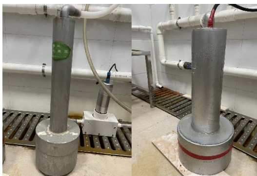
Figure 3. Sputtering degassing device
