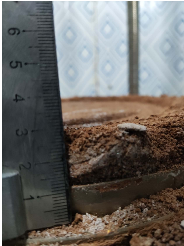
Figure 9. Surface expansion of soil samples 图 9. 土样表面膨胀现象
