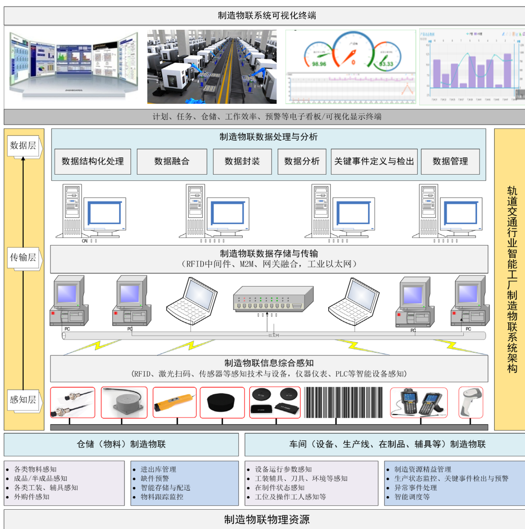
Figure 3. Reference model of Internet of Things system architecture for intelligent factory 图3. 智能工厂制造物联系统架构参考模型
