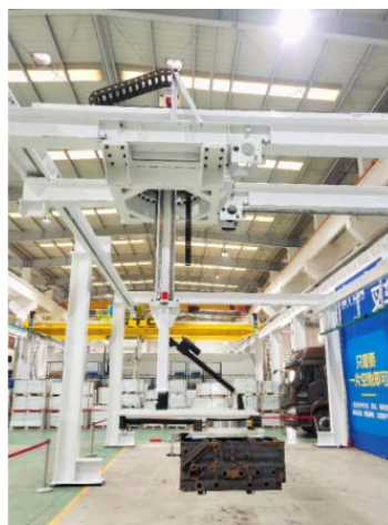
Figure 1. Automatic loading and unloading system of truss robot 图 1. 桁架机器人自动上, 下料系统
