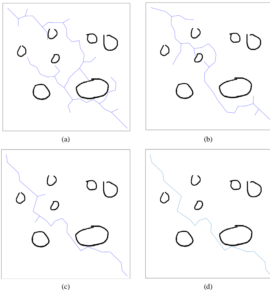
Figure 5. Planning diagram in a simple environment. (a) Conventional BI-RRT; (b) STB-RRT; (c) Trimming STB-RRT; (d) Improved path generation
