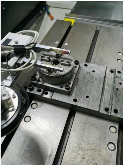
**Figure 2.** The gripper is in the position of the machine tool chuck
