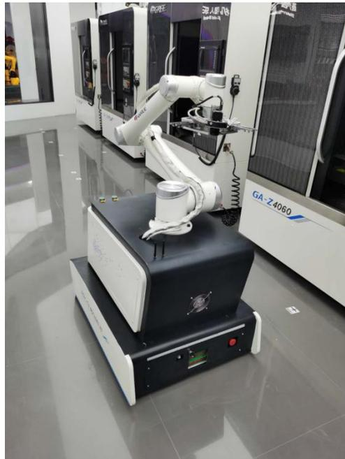
Figure 1. Machine tool collaborative robot and AGV
