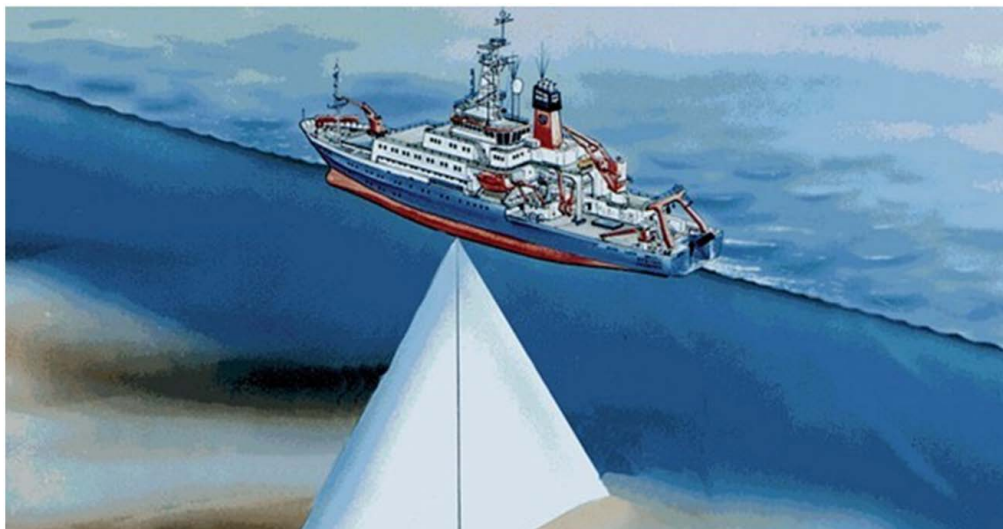
Figure 1. The work sketch of multi-beam sounding system 图 1. 多波束测深系统工作示意图
