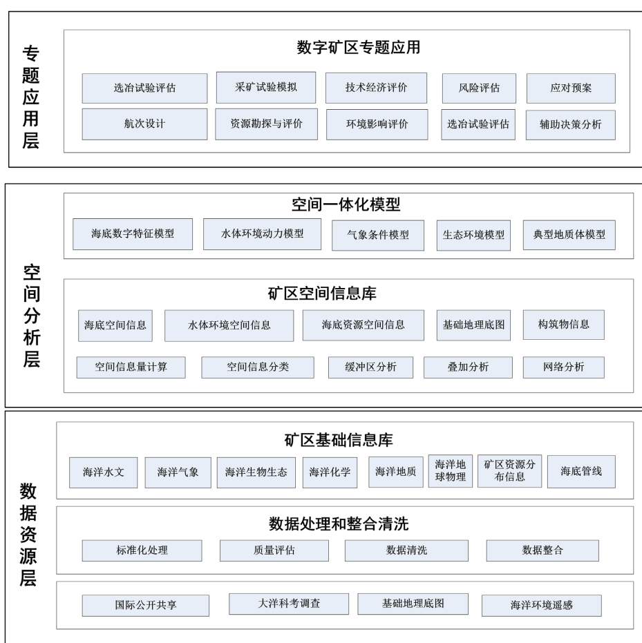
Figure 1. Overall architecture diagram of deep-sea digital mining area construction 图 1. 深海数字矿区建设总体架构图
