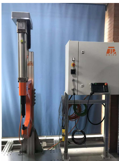
Figure 3. Self-piercing riveting equipment 图 3. 自冲铆接设备
