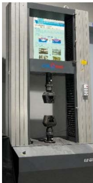
Figure 5. LABSANS LD 26.105 universal testing machine 图 5. LABSANS LD 26.105 万能试验机
