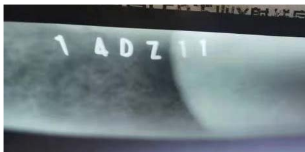
Figure 7. Radiograph of low temperature reheater pipe elbow
