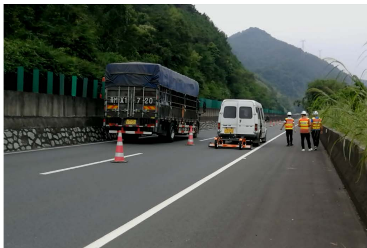
Figure 2. Field work site of 3D radar detection 图 2. 三维雷达探测外业场景
