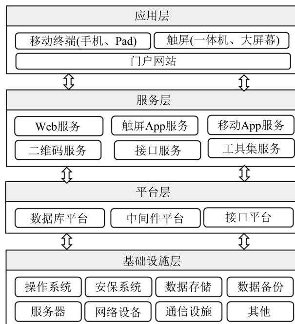
Figure 2. The architecture of the public digital culture cloud service platform
