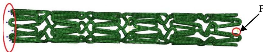
Figure 2. Boundary conditions of the bending simulation of stent. Left end: fixed; Right end: concentrated force 图 2. 支架弯曲模拟的边界条件。左端固定约束，右端中心受集中力作用
