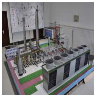
Figure 5. Synthetic ammonia installation model
