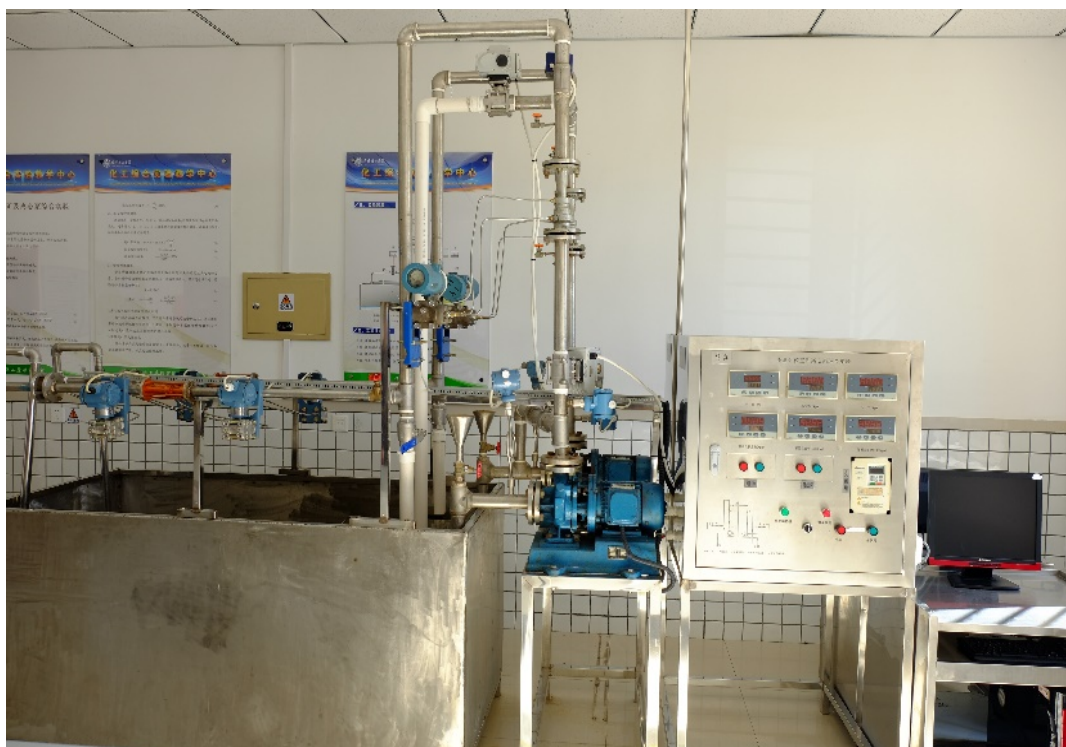
Figure 3. Flow meter correction and centrifugal pump comprehensive experimental device
