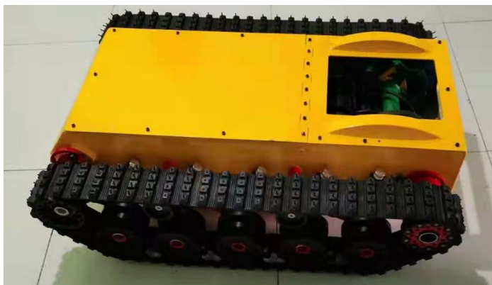
Figure 4. Teaching test prototype car with electric zero differential double flow transmission system
