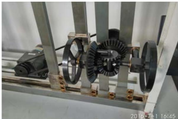
**Figure 2.** Assembled differential system
