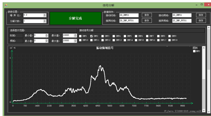
Figure 5. Vibration time frequency conversion result 图 5. 振动时频转换结果显示
