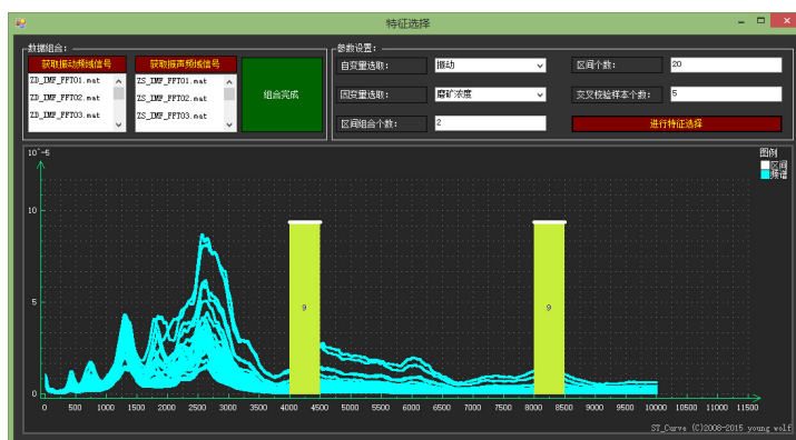
Figure 8. Vibration-grinding concentration characteristic selection 图 8. 振动 - 磨矿浓度特征选择结果显示
