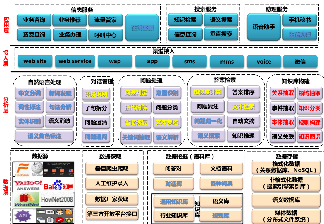
Figure 1. Robot IQA system architecture.
