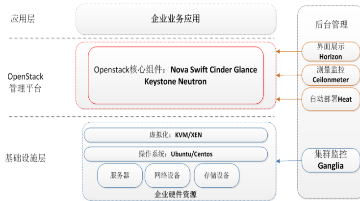
Figure 3. Enterprise private cloud platform system architecture 图 3. 企业私有云平台系统架构
