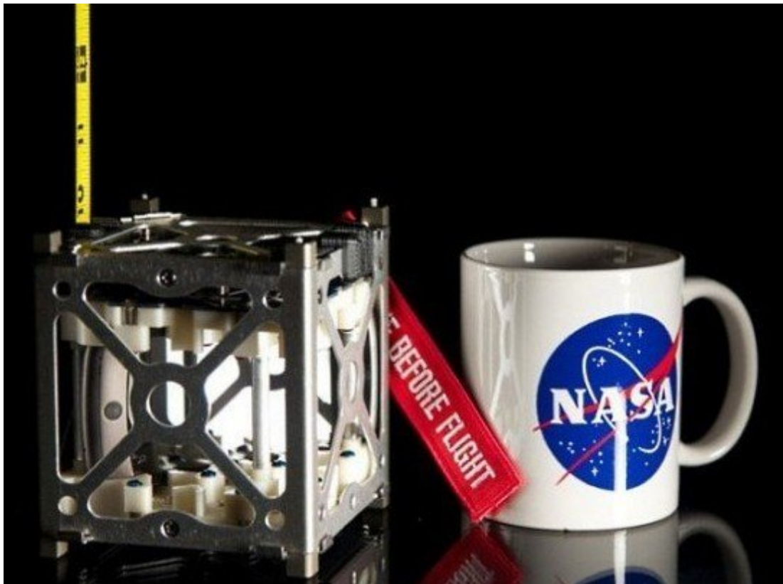
Figure 3. NASA uses micro-system technology to develop a mobile phone satellite, which is the size of a water cup 图 3. 美国 NASA 采用微系统技术开发的手机卫星，仅有水杯大小
