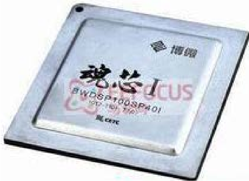
Figure 4. Shows the “soul core # 1” BWDSP100 physical picture 图 4. 国内“魂芯一号” BWDSP100 实物图片
