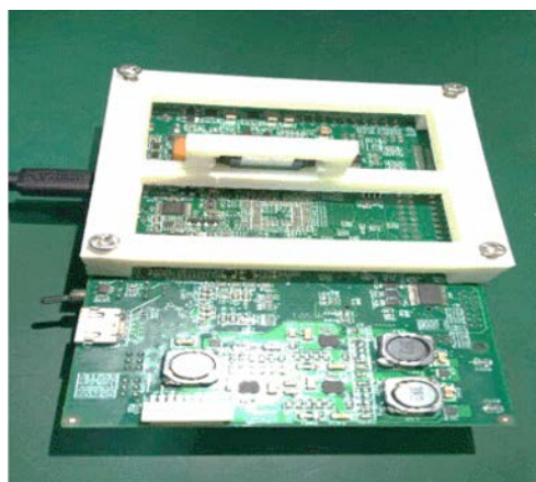
Figure 3. DMD Chip and 3D Printing holder 图 3. DMD 芯片及 3D 打印支架
