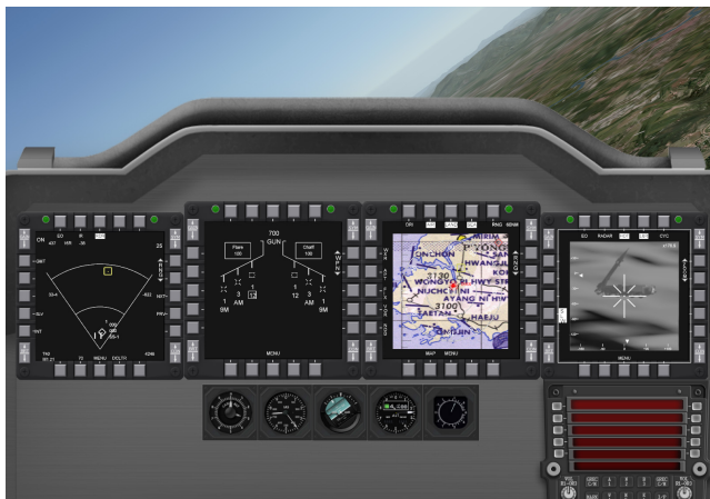
Figure 6. Aircraft virtual cockpit constructed by GLS virtual instrument in OSG environment
