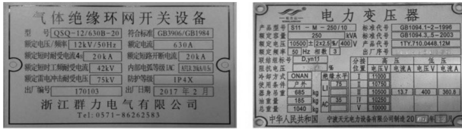
Figure 12. Nameplate of electrical equipment 图 12. 电力设备铭牌
