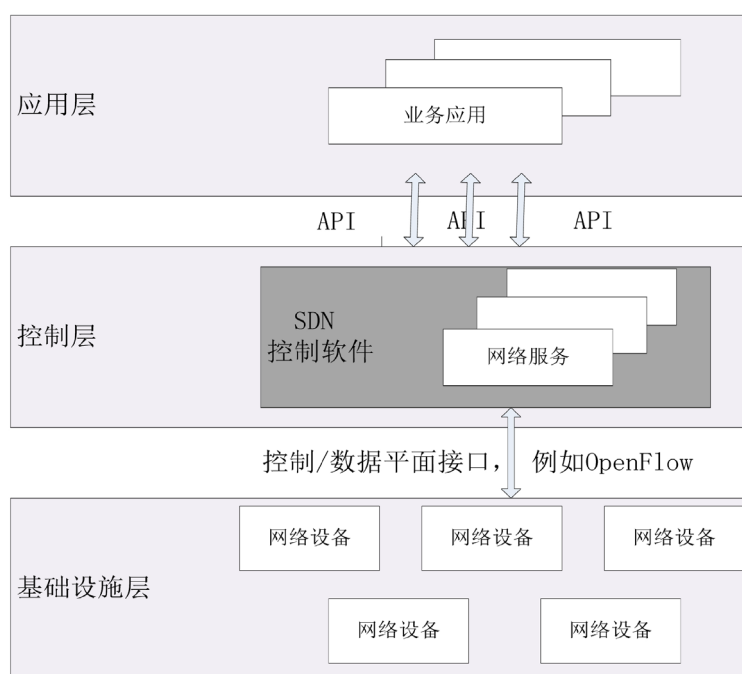
Figure 1. The basic architecture of SDN
