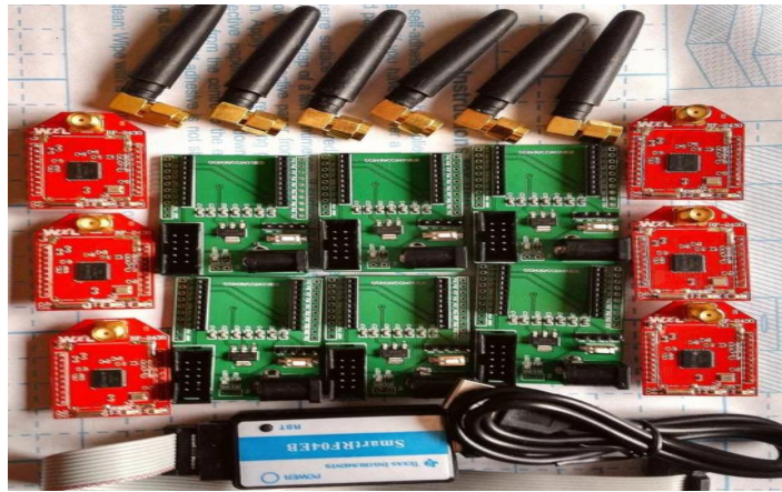
Figure 1. The hardware used in the system (CC2430 and CC2431 modules, emulator)
