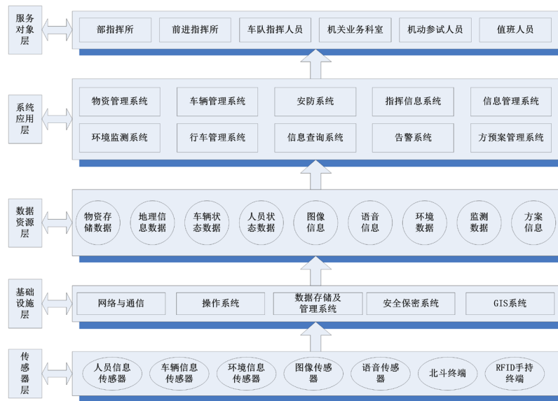
Figure 1. Architecture of integrated support system for mobile delivery informatization 图 1. 机动投送信息化综合保障体系架构图
