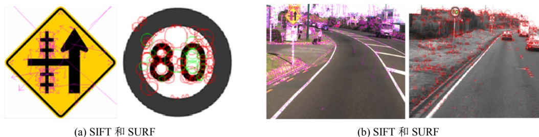
Figure 2. SIFT and SURF features extracted 图 2. SIFT 和 SURF 特征提取
