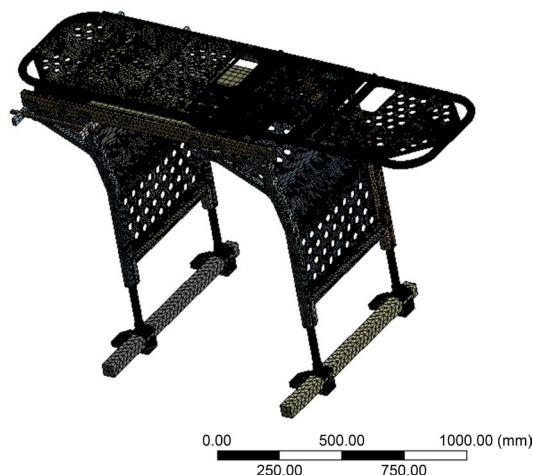
Figure 1. Finite element model of aircraft stretcher
