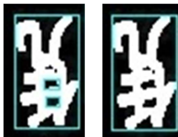
Figure 3. Comparison of the effect of non-maximum suppression algorithm before and after processing 图 3. 非极大值抑制算法处理前后效果对比图
