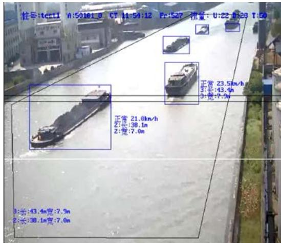
Figure 5. Length and width of ship
