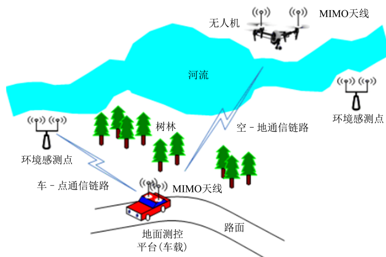
Figure 2. The working process of the wireless broadband data transmission system 图 2. 无线宽带数据传输系统工作过程示意
