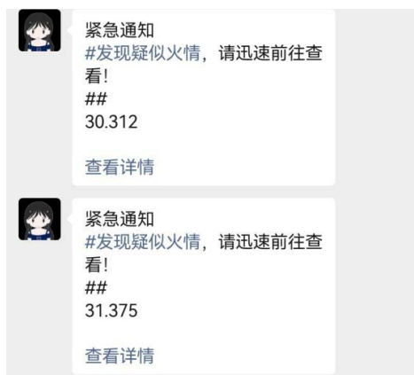
Figure 3. Message notification received by mobile phone (over 1 degrees Celsius warning within 1 minute)
