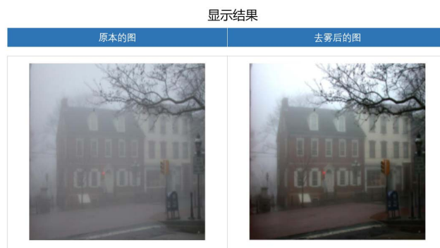
Figure 4. Dark channel guided filter defogging effect
