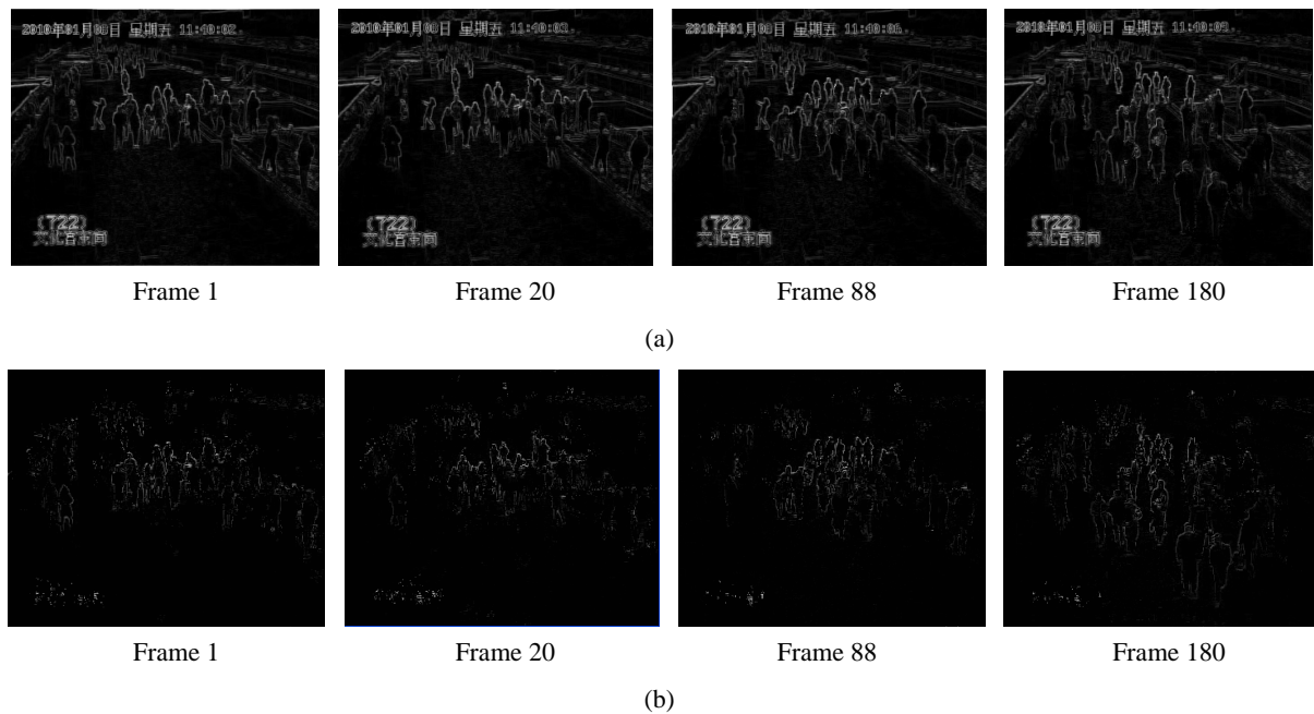
Figure 2. The effect of improved Kalman filter algorithm. (a) The effect of background update; (b) The effect of crowd recognition
