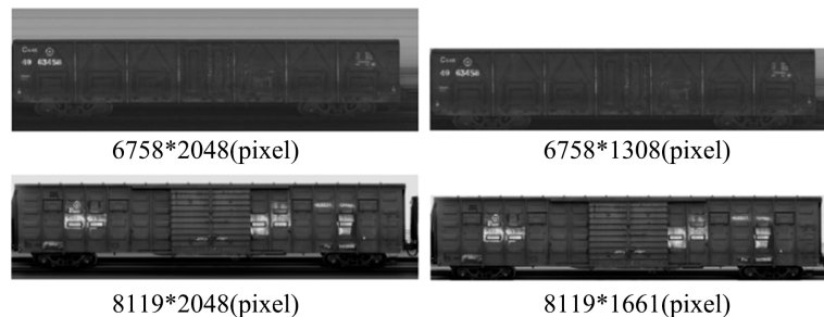
Figure 5. Comparison of line array image before and after segmentation 图 5. 线阵图像分割前后的对比图
