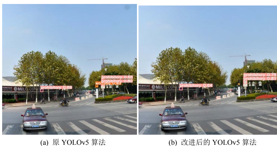
Figure 6. Traffic sign detection renderings before and after improvement (2) 图 6. 改进前后交通标志检测效果图(2)
