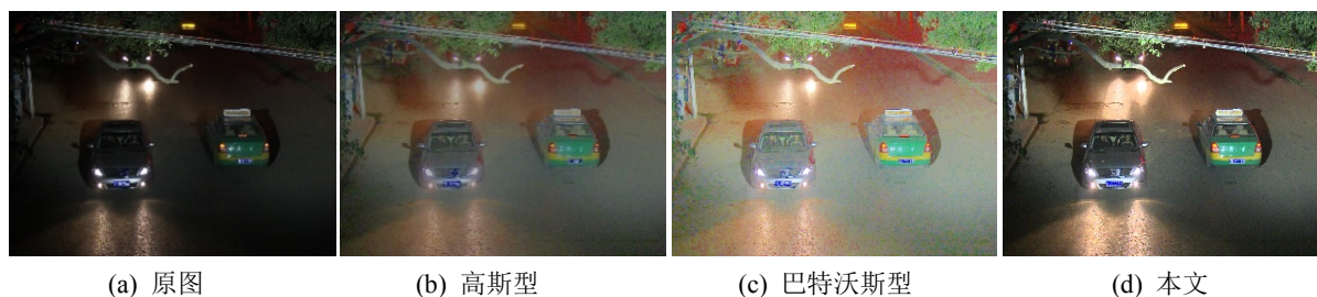
Figure 5. Comparison of road image enhancement effect 图 5. 道路图像增强效果对比
