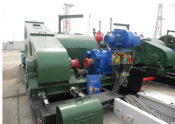
Figure 1. Asynchronous motor mud pump system 图 1. 异步电机泥浆泵系统
