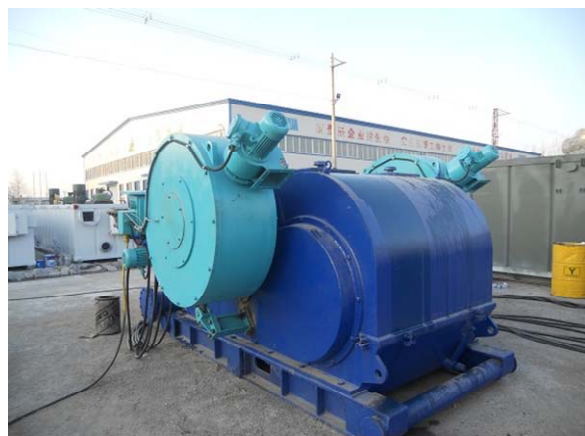
Figure 2. Double motor coaxial control system for mud pump assembly site in Liaohe oilfield 图 2. 辽河油田双电机同轴泥浆泵装配现场
