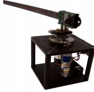
Figure 1. The models of SRV02 and the Rotary Flexible Link 图 1. SRV02 模块和 Rotary Flexible Link 模块
