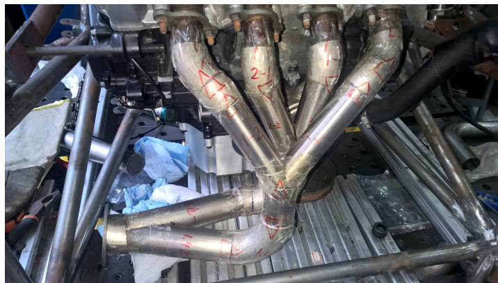
Figure 12. The exhaust system is completed 图 12. 一二级歧管搭建完成
