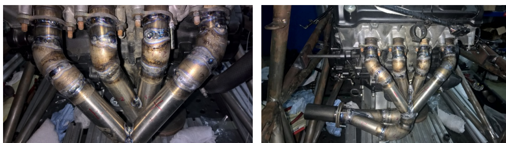
Figure 14. Exhaust system welding completed 图 14. 焊接完成的排气总成
