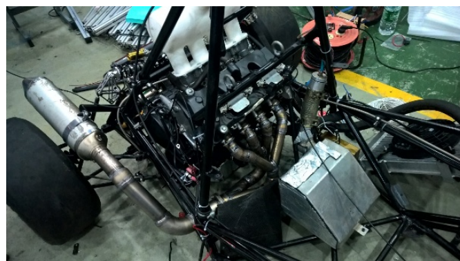
Figure 15. Exhaust system installation completed 图 15. 排气系统在赛车上的安装
