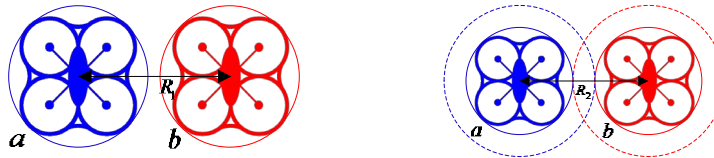
Figure 2. (a) Minimum safety distance; (b) Collision avoidance distance
