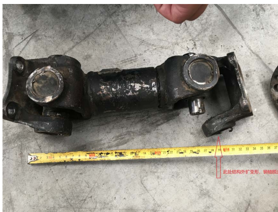
Figure 22. Failure of the drive shaft 图 22. 传动轴失效现象
