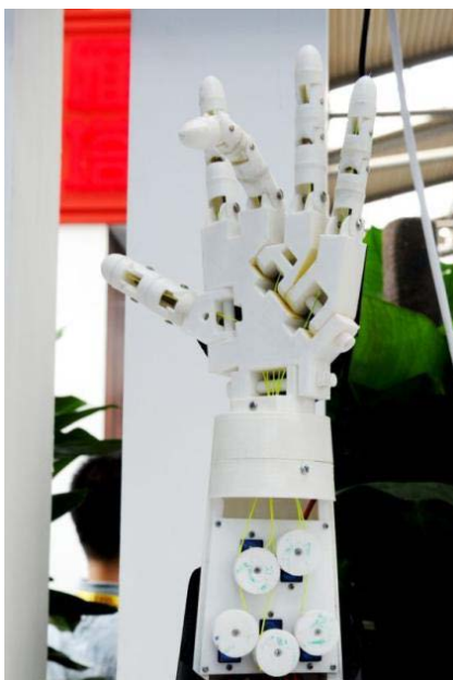
Figure 1. Five-finger manipulator with rope driven
