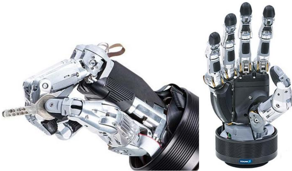
Figure 7. Five-finger manipulator with joint motor 图 7. 关节电机驱动型五指机械手
