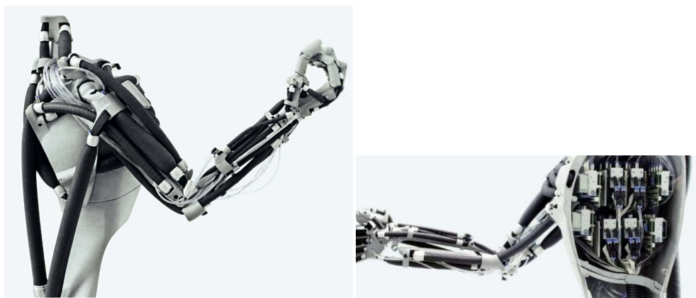
Figure 6. Five-finger manipulator with highly integrated pneumatic muscle 图 6. 高度集成化的气压驱动五指机械手
