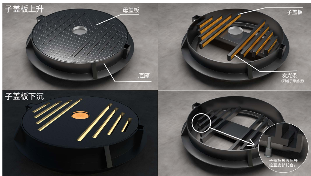
Figure 10. Structure diagram of automatic opening and closing manhole cover 图 10. 自动开合式井盖结构图 ⑫
