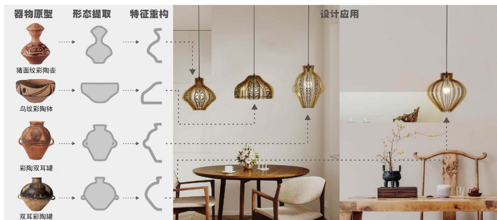
Figure 5. Design of Yangshao colored pottery series luminaires 图 5. 仰韶彩陶系列灯具设计 ①
