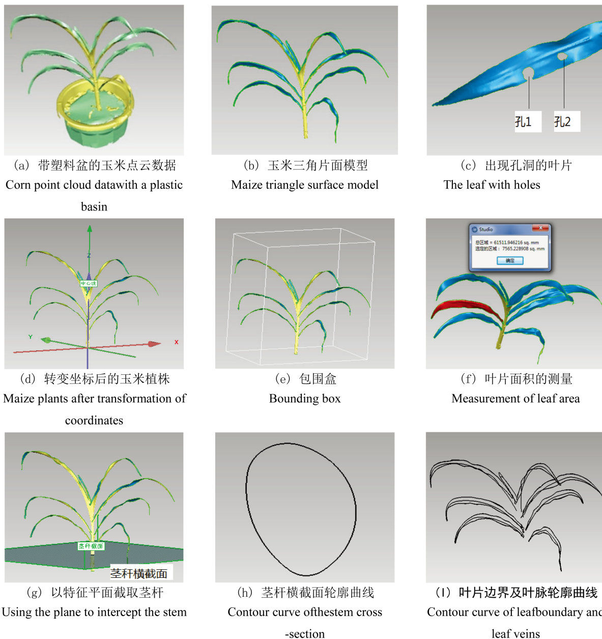
Figure 3. Point cloud data processing and acquisition of morphology index 图 3. 点云数据的处理及形态指标的获取
