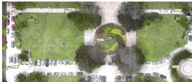
Figure 3. Aerial survey area SfM three-dimensional reconstruction 图 3. 航测区 SfM 三维重建
