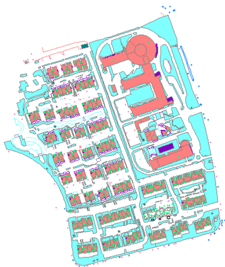
Figure 4. Finished topographic map results in the test area 图 4. 试验区内竣工地形图成果
